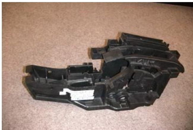
Torque converter bracket PP LGF 40 %
