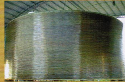
Total filament-wound finished.
